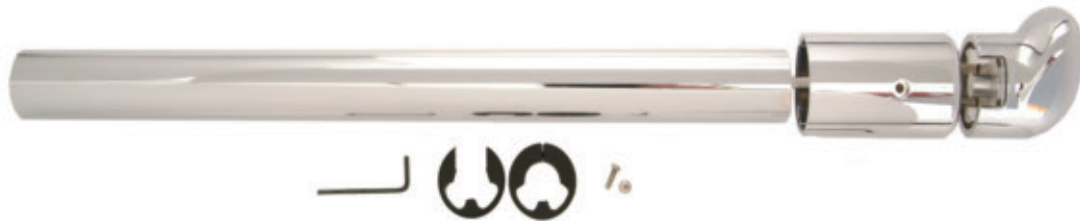
UST323 Shift Lever Cover Assembly Set - Complete w/Billet Alluminum Chrome Knob (accommodates range selector and splitter), Chrome Plated Shift Lever Cover Skirt & Sleeve Set
