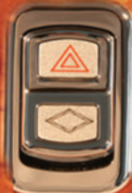
PP-27HA Hazard Lights
